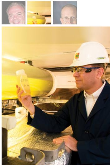
Clayton McNeff holds up a bottle of biodiesel produced with waste cooking oil at the Mcgyan Biodiesel pilot plant. The Mcgyan process has been used to convert many oils including corn oil, to biodiesel.
